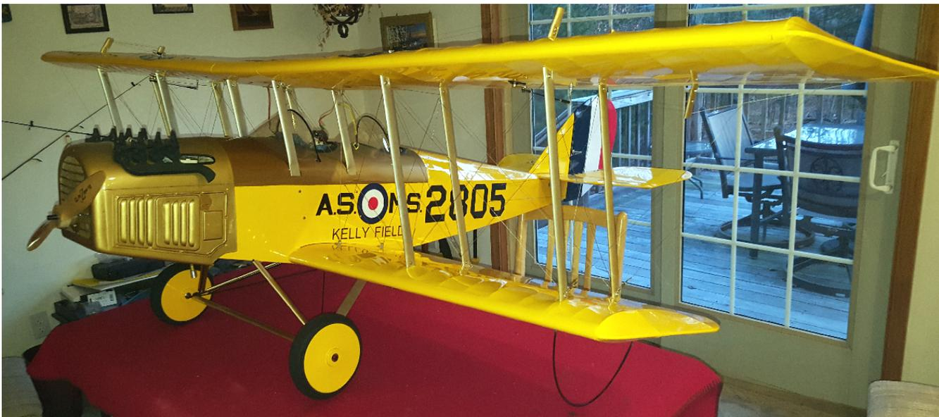
The prop is going to be a Jack Mertz 24 x 6-10 replacing the 22 x 10 used on the Wyvern. The throttle and choke servos are mounted on the engine box and covered with self adhesive heat reflective tape. The metal coating should help to reduce stray RF ignition noise from entering the Rx system.
